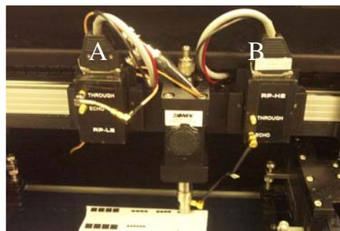
Figure 2: High frequency PE/TT configuration
