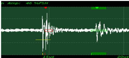
Figure 5: The combined pulse-echo (red gate) and through-transmission signal (green gate)
