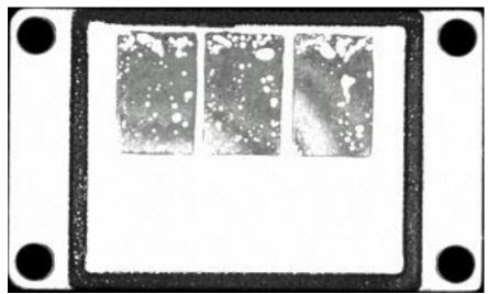
This is a pulse-echo (reflected) mode image of bond quality between a solder pre-form prepreg and a coppertungsten base plate. Voiding in the solder bond can be seen. Studies have shown that die temperature becomes critically high when solder layers become greater than 25% disbonded. In addition, disbonds and voids have been shown to expand upon
