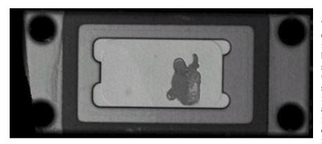
This is a pulse-echo (reflected) mode image of bond quality between a die and the substrate. Voiding in the solder bond can be seen as white in this image. This device also suffers from insufficient solder coverage over the intended bond area.
