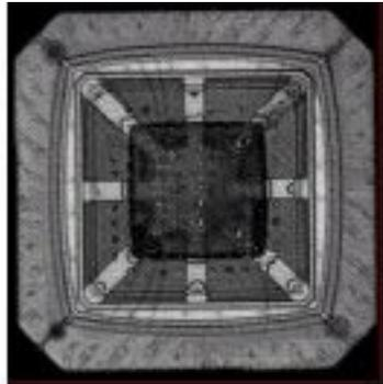
This is a pulse-echo (reflected) mode image of a Ball Grid Array package. A 75MHz 12mm focal length transducer created this image. This peak amplitude TAMI™ Scan image shows all four layers of primary interest in this BGA. Bright white areas in the upper left image represent disbonds between the encapsulant and die. Disbonding on the top of the die will cause the bond wires to not make an adequate electrical connection. Disbonding can also be found between the die attach and heat
