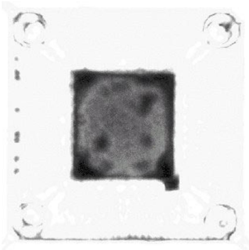
This through transmission mode C-scan image was taken using a 15MHz transducer. A 15MHz transducer was used on the same PLCC package seen previously. Black areas on the image confirm the delaminations seen in both of the previous pulse-echo images.
