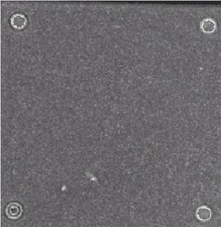
This pulse-echo C-scan image, taken using a 15MHz transducer, is of the molding compound of a PLCC package. Called a Material Scan, several locations of air voids trapped within the encapsulant material can be seen as white circular areas. Particle and density variations within the encapsulant can also be seen.
