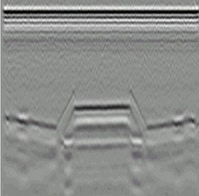
This pulse-echo B-scan image, taken using a 15MHz transducer, show a non-destructive cross-section of the x-z plane of a PLCC package. It can be seen in this image that the die is tilted within the package relative to the front surface of the package. Die tilt is frequently caused by either misplacement/alignment or forces exerted upon it from the thermally-induced expansion of the materials surrounding it.
