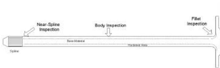
Figure 1: Rear Axle Cross Section showing typical ultrasonic inspection points to measure case depth.
