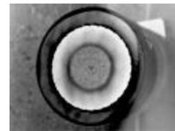
Figure 2: Cut, polished and etched cross-section showing hardened outer region and soft core on a hardened axle.
