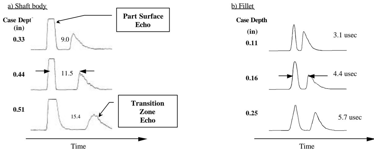
Figure 3: Ultrasonic responses from: (a) 3 shaft bodies having case depths of .33, .44, and .51 inches, and (b) three fillets having case depths of 0.11, 0.16, and 0.25 inches.
