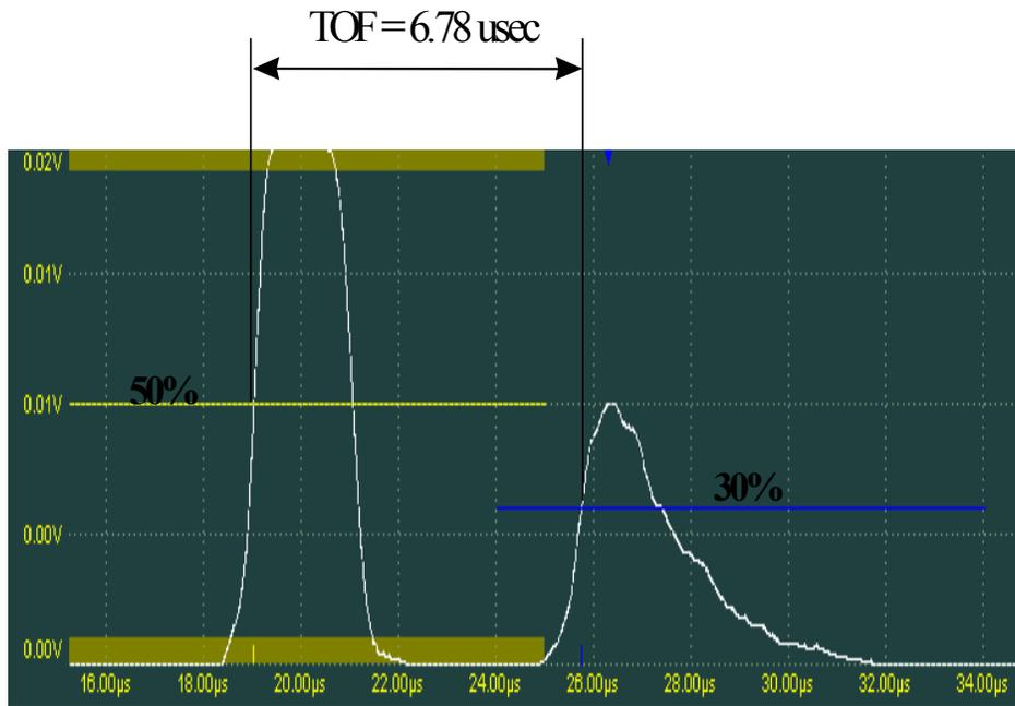
*Figure 2: Time-Of-Flight Measurement (TOF) between “Front-Surface” and “Transition Zone” reflections.*
