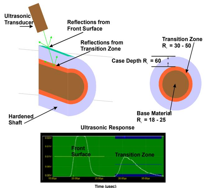
Figure 1: Ultrasonic response from a hardened steel axle shaft.
