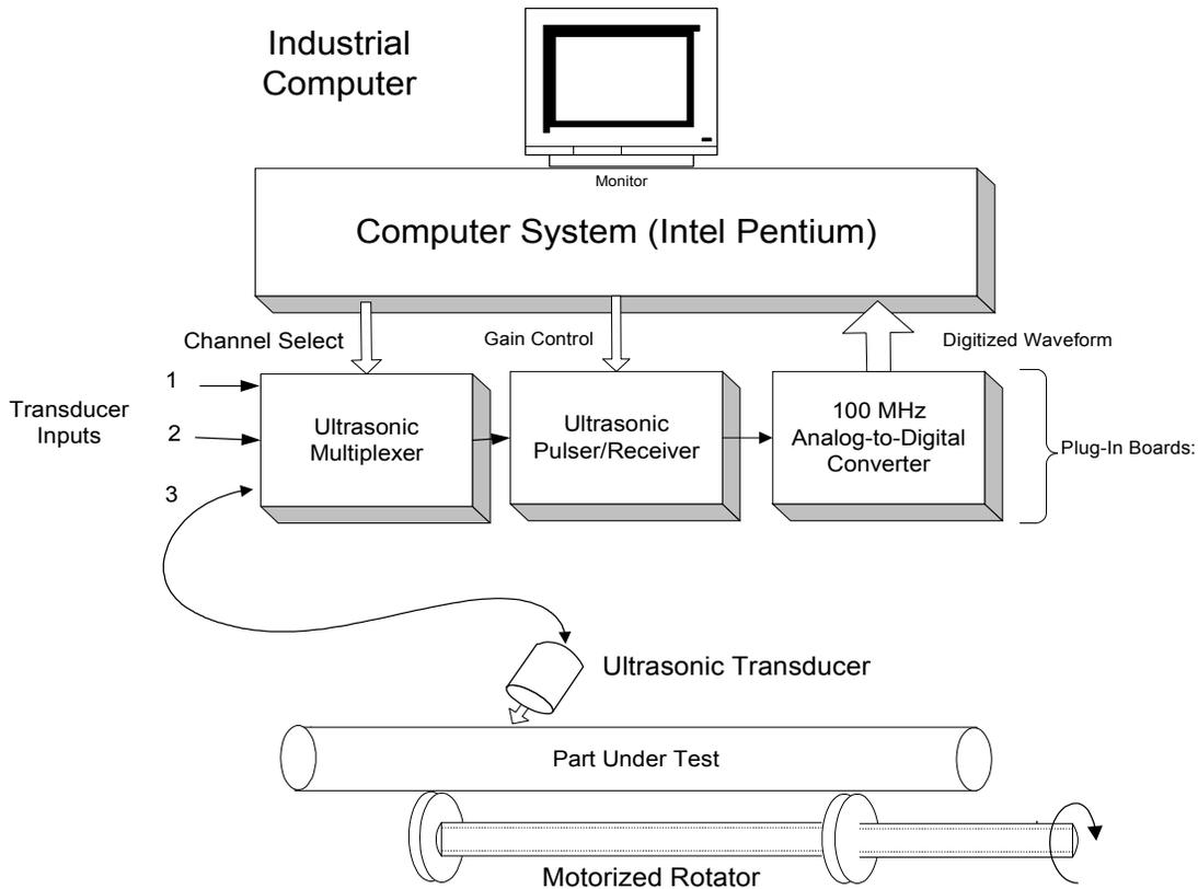
*Figure 5: Simplified Block Diagram of UMA System.*
