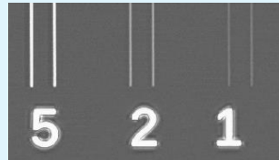
Zoomed in SAM image of the line defect pattern showing detection of 1µm line width defects
